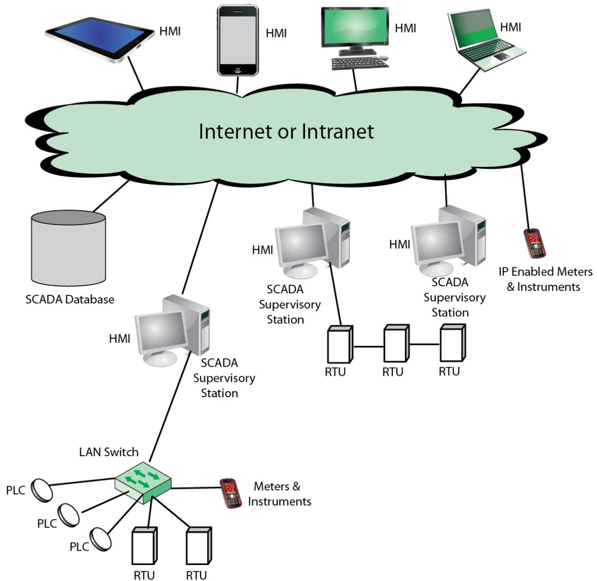
Figure C6.1 SCADA Example
